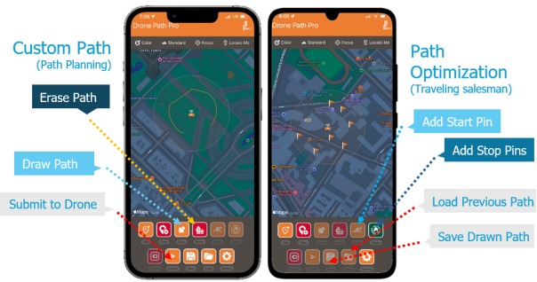
Fig. 3. Mobile Device UI for Drawing and Path Optimization.
